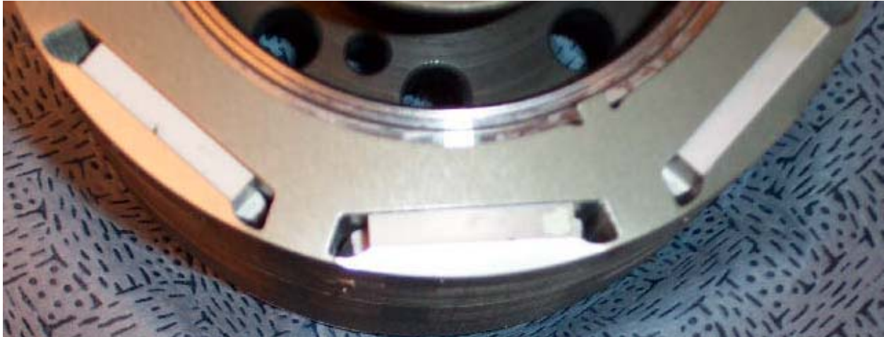
Figure 5 – Toyota Prius permanent magnets (Source: ORNL [4] )
