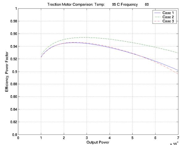
Figure 3: Comparison of operating efficiencies at 60 Hz
