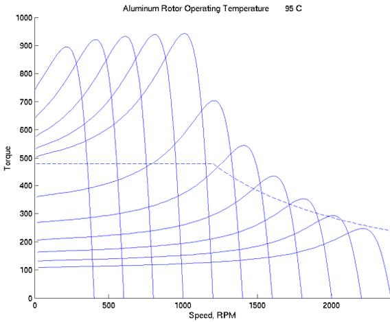
Figure 8: Capability of the Aluminum Rotor Machine
