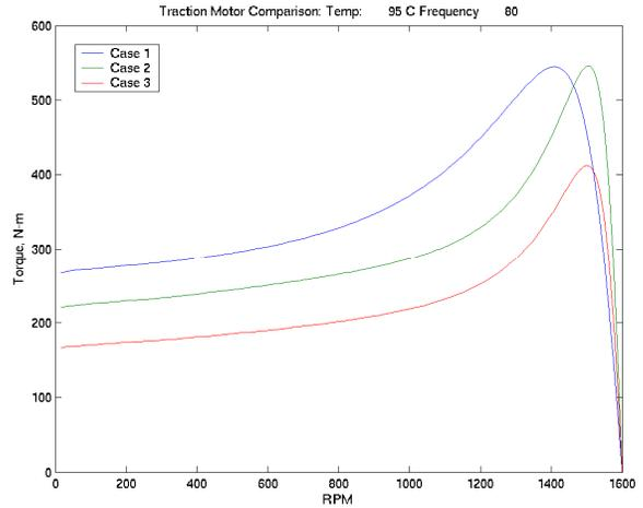
Figure 6: Comparison of Torque at 80 Hz
