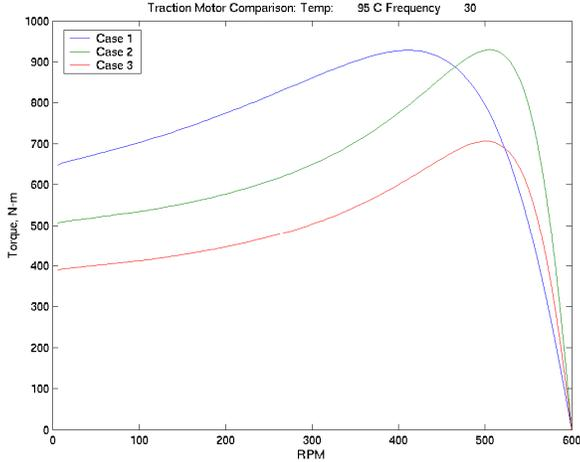
Figure 4: Comparison of Torque Speed Curves at 30 Hz.
