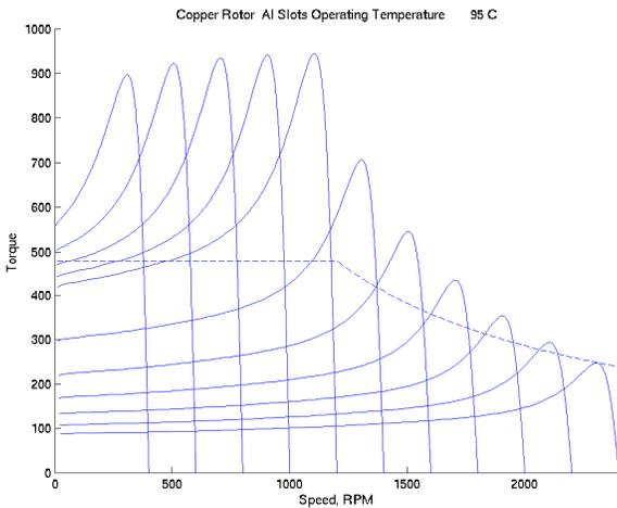
Figure 9: Capability of Copper Rotor Machine in Aluminum Slots
