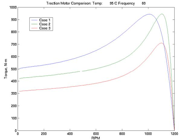
Figure 2: Comparison of Torque-Speed Curves at 60 Hz:
