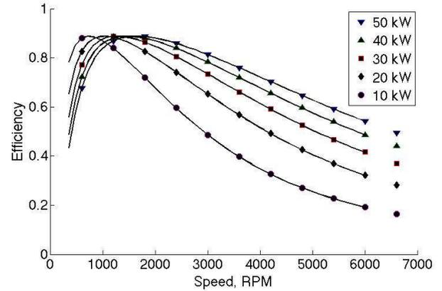
Figure 5 - Estimated efficiency of PM Machine
