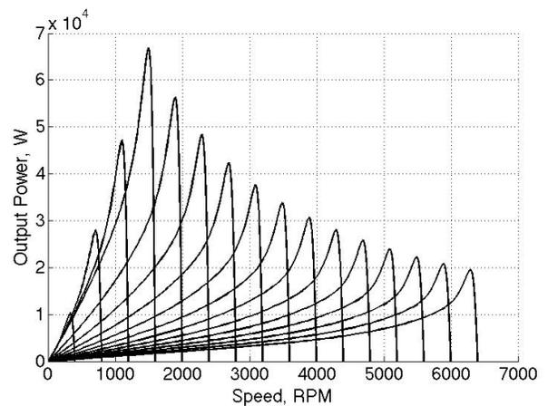
Figure 3 - Power Capability of Induction Machine with Cast Copper Rotor
