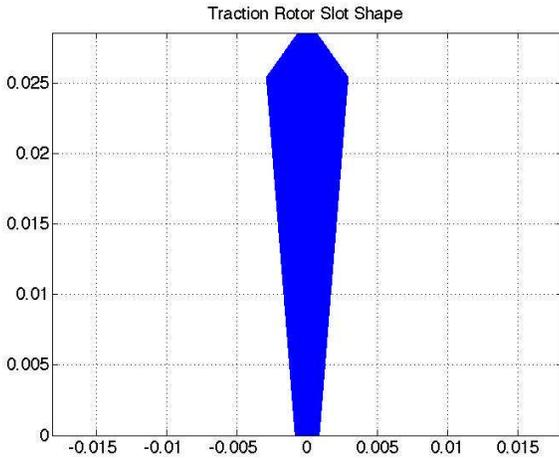
Figure 1- Traction Motor Bar Shape
