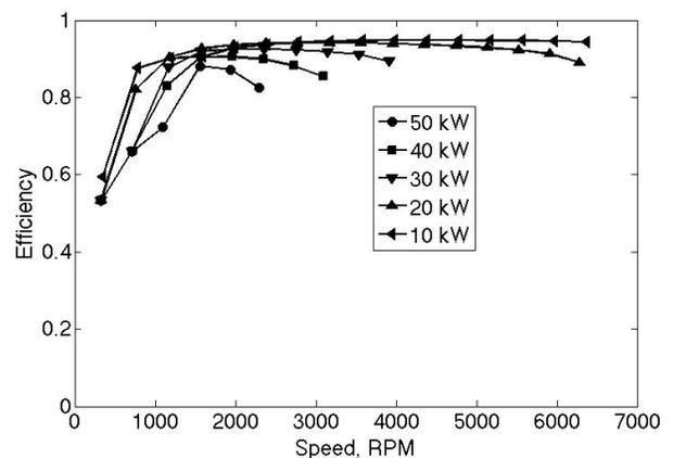
Figure 4 - Efficiency of the Induction Machine with Cast Copper Rotor
