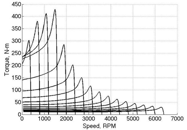
Figure 2 - Illustration of Torque Capability of Induction Machine with Cast Copper Rotor
