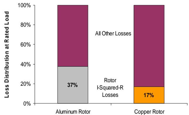
Figure 11 - Loss distribution at rated load showing dramatic reduction in rotor conductor loss with the optimized die cast copper rotor design.
