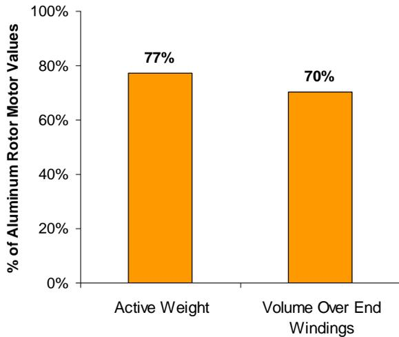
Figure 9 - Relative Weight and Size of the Die-cast Copper Rotor Motor Compared to the Aluminum Rotor Motor
