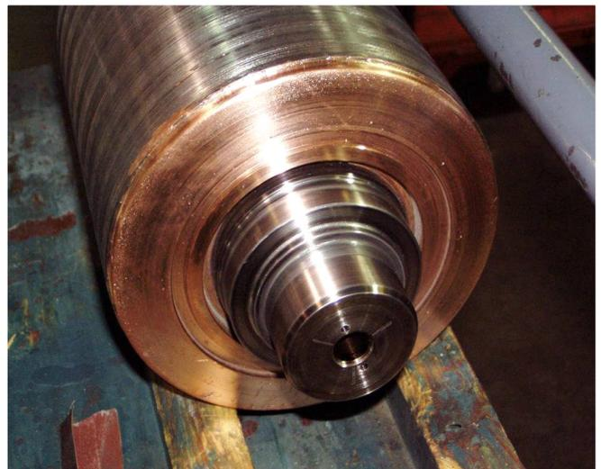
Figure 14 - Copper die cast rotor for the traction motor application.
