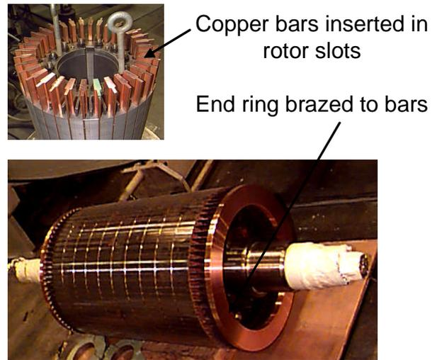
Figure 13 - Fabricated copper bar rotor using traditional copper rotor manufacturing techniques.
