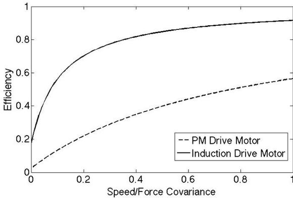
Figure 8 - PM Drive Effective Efficiency
