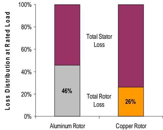
Figure 10 - Loss distribution at full load for the traction motor designs showing a much smaller portion of the motor loss is in the rotor for the copper die cast rotor motor.
