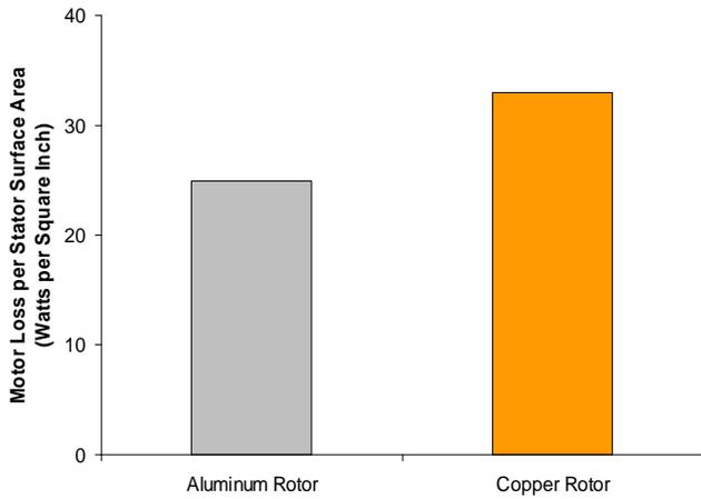
Figure 12 - Total motor loss per stator surface area showing significant improvement with die cast copper rotor design.
