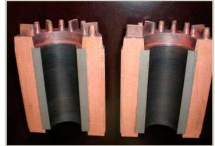
*Cross-section through Rotor Bars and End Ring of Die Cast Copper Motor Rotor*
