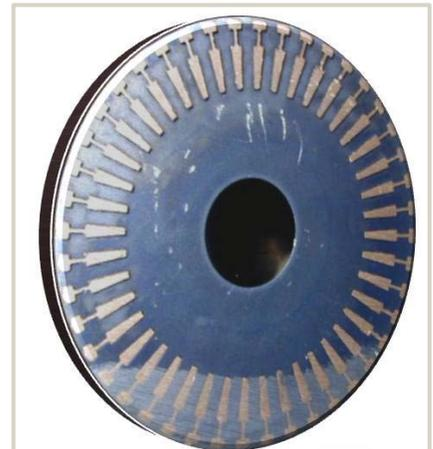
*Cross-section through Rotor Bars of Die Cast Copper Motor Rotor*
