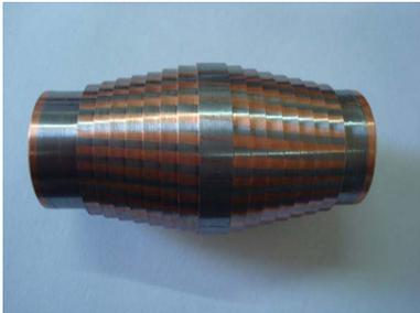
Fig. 4. Quality of cast copper rotors in different diameters and lengths
